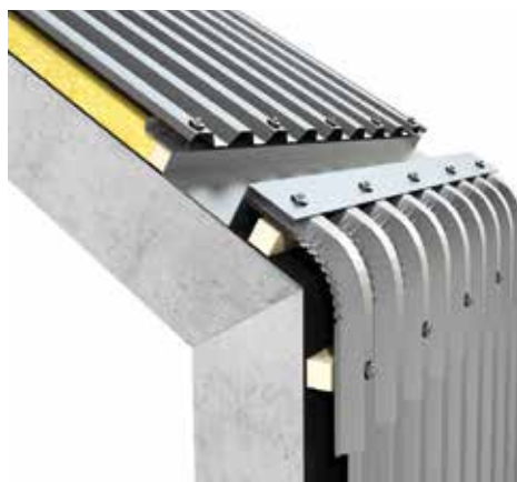
RACCORDO CON PARETE JOINT BETWEEN ROOF AND WALL
