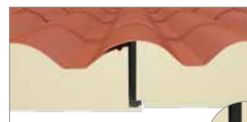
Sovrapposizione laterale mezza onda Side overlap of half a corrugation
