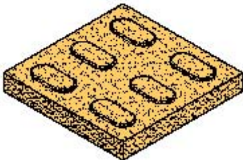
On-Street Warning Paving
